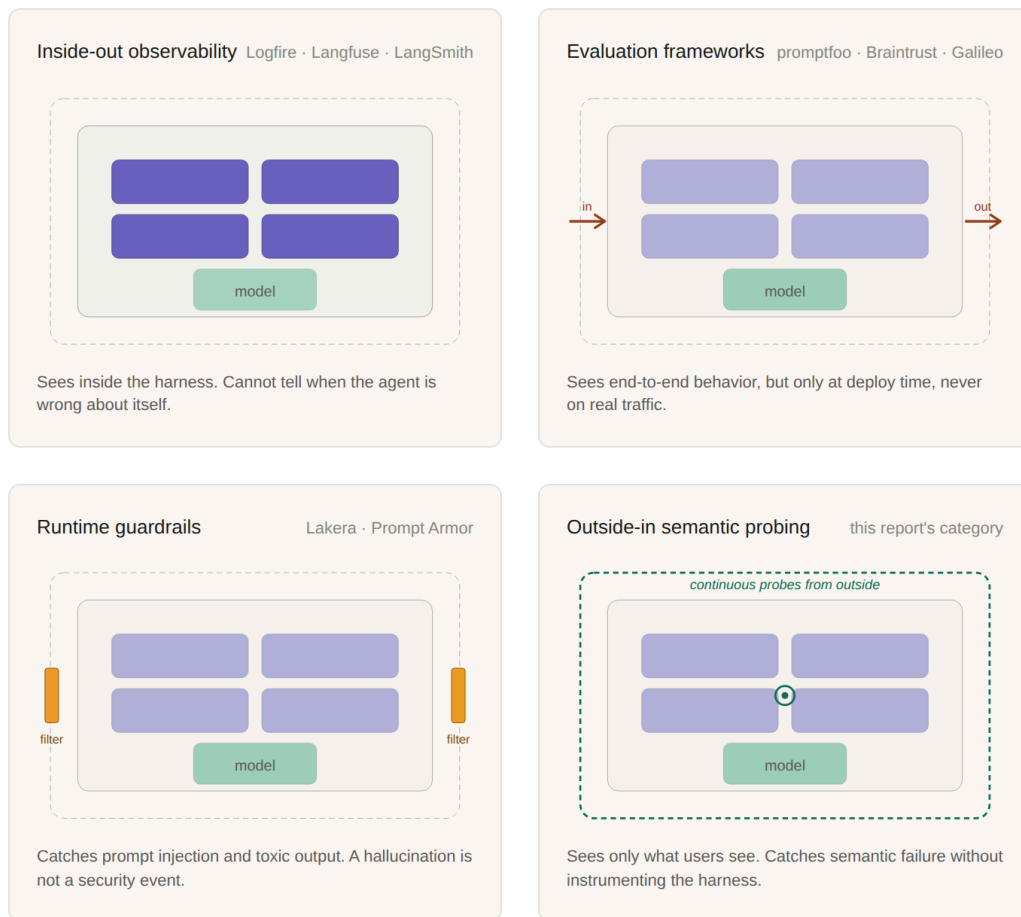
Figure 6. Where each existing monitoring category looks on the agent's model and harness. Inside-out observability instruments specific harness regions. Evaluation frameworks run inputs through the whole agent but at deploy time. Runtime guardrails screen the perimeter for security threats. The category this report argues for sits entirely outside the agent, probing continuously from the user's vantage point with no instrumentation of any harness region.
